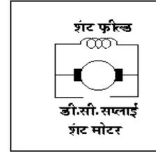
Applications- e.g. pump, lathe m/c, drill m/c, printing m/c, etc.
