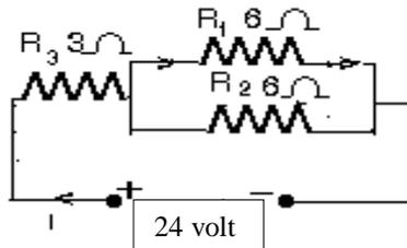
First calculate total resistance of parallel circuit  $R = \frac{R_1 \times R_2}{R_1 + R_2}$
