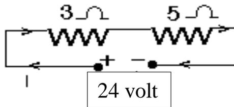
Total resistance of the circuit  $R = R_1 + R_2$  where  $R_1 = 3\Omega$  and  $R_2 = 5\Omega$
