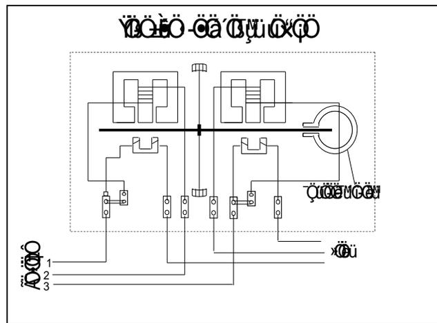
**Construction** In this meter two coils are placed on one core as shown in the picture. Current coil made up of less number of turns of thick wire. Pressue coil is of more number of turns with thin wire. Disc rotates due rotating field created by current coil and pressure coil. These are placed at electrically 90 degrees apart.
