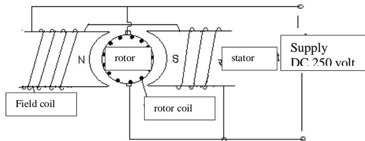
When supply is given to both of these windings, due to current stator and rotor field is established. Direction of field is as per the direction of current. Due to effect of these field force is acted upon a rotor and it rotates.
