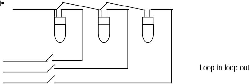
**2. T wiring-** in this type phase is taken through switches and neutral through bulb holders.
