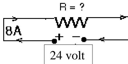
Resistance of the circuit =  $\frac{\text{Voltage}}{\text{current}}$
